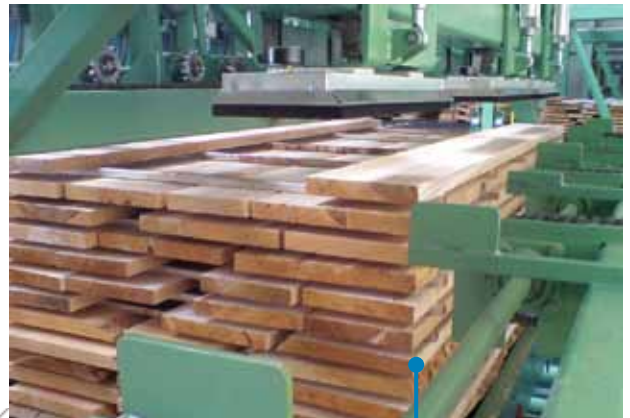
Automatic layer formation with suction robot
