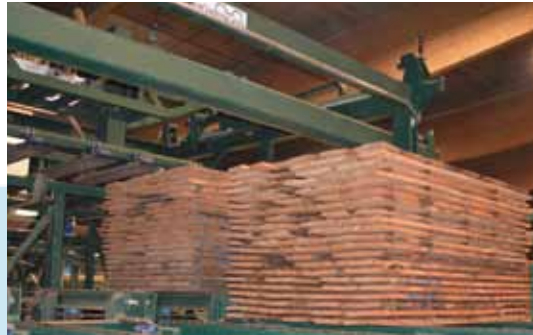
Destacking of packs and removal of stickers
