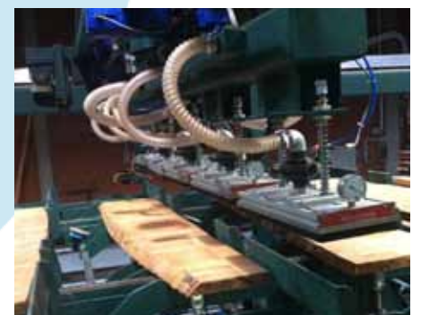
Board selection out of an intermediate buffer with a vacuum robot
