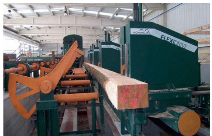
Precise fixation for longer logs
