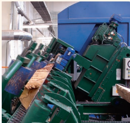
Inclined execution for automatic separation
