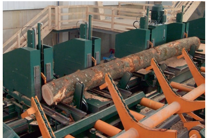
FLEXIDRIVE with hydraulic log turner
