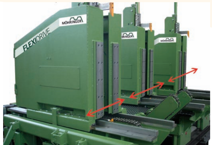
Each clamping head longitudinally movable
